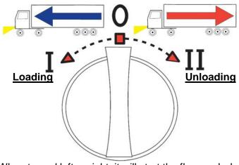
When turned left or right, it will start the floor and when released it will automatically return to the 0 position
