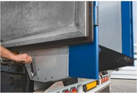
Before mounting one must determine at which spot enough room is available in order to mount the roll. With most bodywork this is possible directly under the rear portal of the trailer. Pay attention to that you do not cover the lights.
