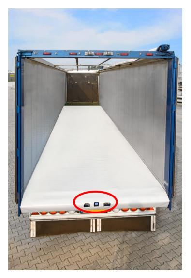
Roll the protection sheet fully out to the headboard of the trailer. If necessary it can be shortened on the headboard side and equipped of a loop for the tube ø 20 mm. Holes must be cut into the sheet at the position of the locks of the doors. The doors can then be locked while the protection sheet is rolled out over the floor.
