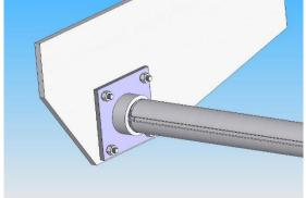
When the position is determined one can start with mounting the mounting plates onto the rear portal. Pay attention to that the axle is hanged horizontally comparatively to the floor of the trailer.
