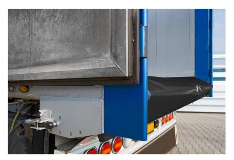
A connection must be made to the accessory air circuit if you have a pneumatic roll mechanism for the protection sheet. After this the two position valve must be mounted on the chassis so the driver can simply operate this valve nearby and can supervise the unloading
